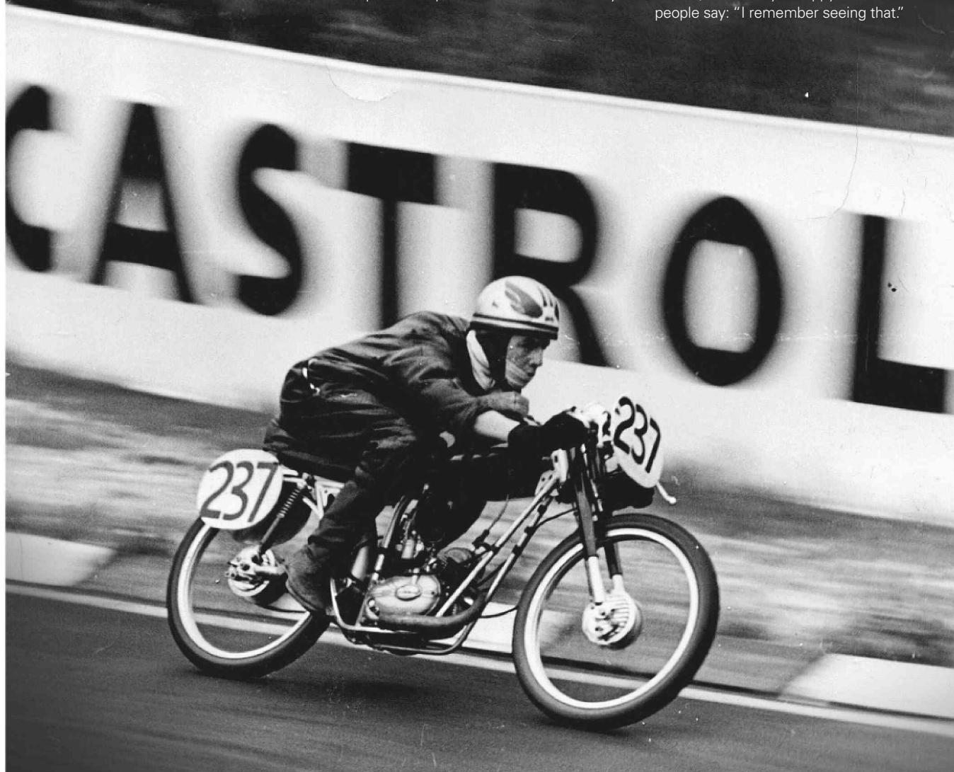
Early days with the air-cooled Demm, no pumped gearbox oil and undamped suspension units. Believed to be taken at Brands Hatch, at Bottom Bend
