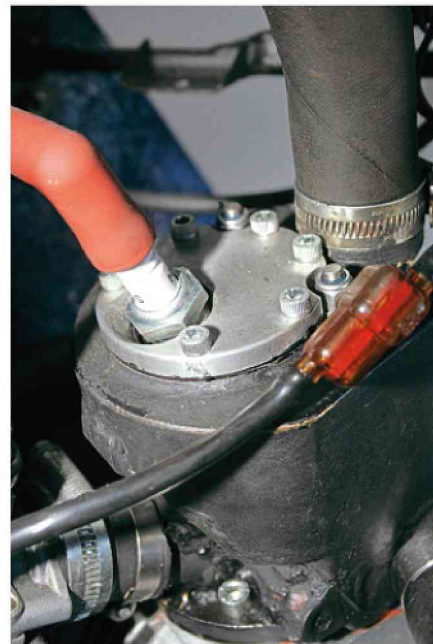
Above: The cylinder head skull and squish band could be changed without disturbing the water jacket
